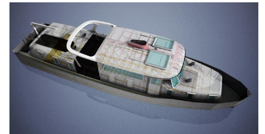
superstructure with the hull framing partially visible
